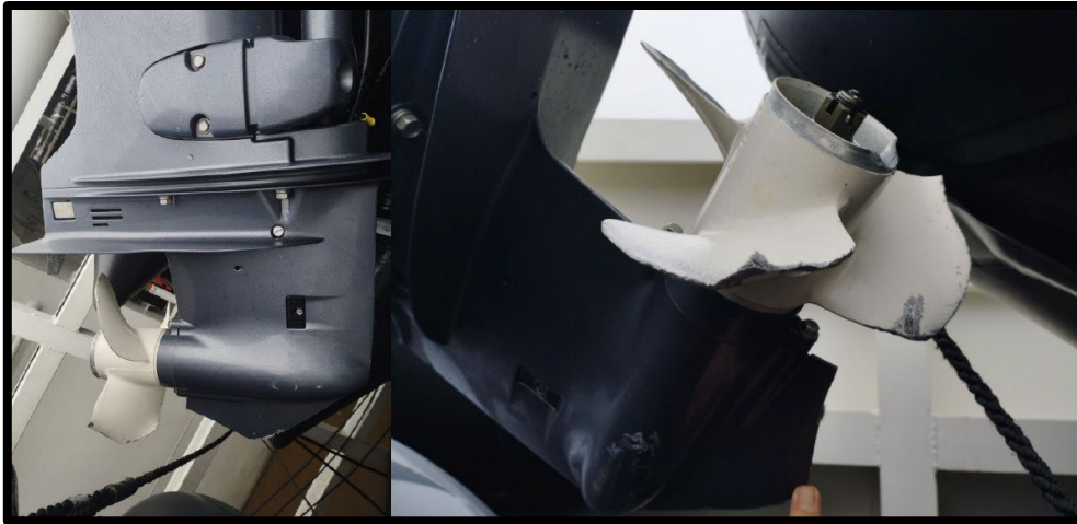
Figure 9 – Photos of damaged propeller on Zodiac #4 (provided by Quark Expeditions)
